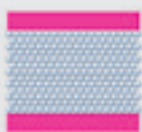
Arrangement of the Vacuform® 2.0 MicroSpace balls without vacuum
